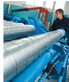
Spiral wound ducts workshop
